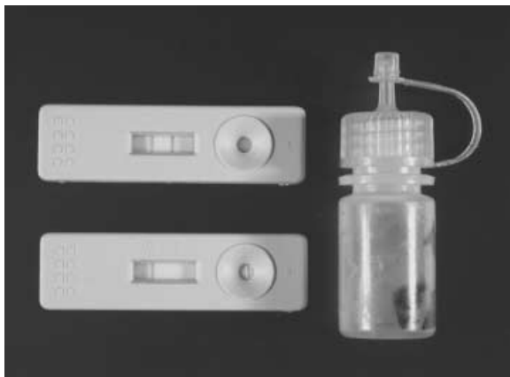
Figure 1 Lateral flow devices (positive result: upper LFD; negative result: lower LFD) and extraction bottle.
