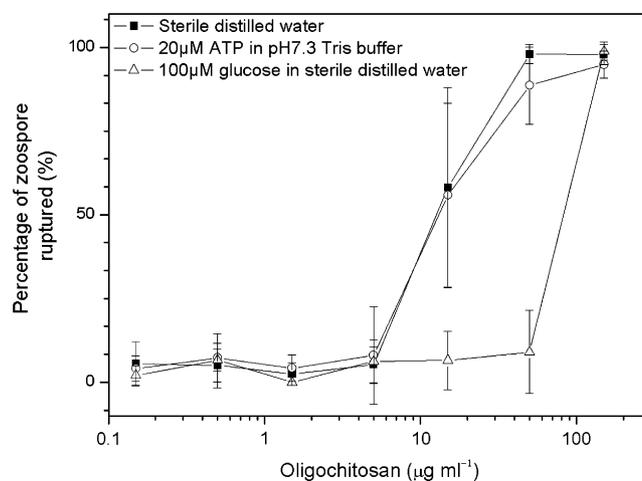
Fig. 4. Effect of glucose on zoospore rupture caused by oligochitosan. 100 mM glucose in sterile distilled water was added 10 min before addition of oligochitosan. Zoospore rupture was measured after 60 min incubation.
